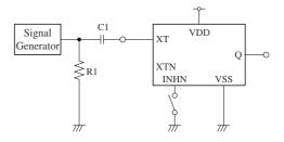
2Vp-p, 10MHz sine wave input signal C1: 0.001µF R1: 50Ω
